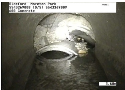
i. CCTV images showing collapsed culvert and a ground level image taken of the sinkhole.
